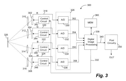
Figure 3 depicts digital camera 300. *Id.* at 4:62–64. Digital camera 300 includes lenses 310, 312, 314, 316. Each lens has a corresponding imaging sensor 302, 304, 306, 308. *Id.* at 4:64–67. Each imaging sensor is integrated with a transmissive filter. *Id.* at 5:14–17. In the preferred embodiment, imaging sensor 302 uses a red filter, imaging sensor 304 uses a green filter, and imaging sensor 306 uses a blue filter. *Id.* at 5:17–21. Imaging sensor 308
