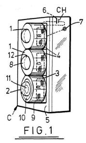
Figure 1 depicts a video camera system having three cameras 1, each comprising lens system 2 mounted on image sensing surface 3 of image array sensor 4. *Id.* at 9:20–28.
