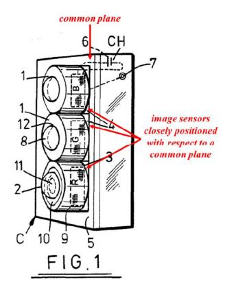
Annotated Figure 1 depicts a video camera system having three cameras 1, each comprising lens system 2 mounted on image sensing surface 3 of image array sensor 4 with annotations identifying the image sensors and their relative positions with respect to a common plane. Ex. 1008, 9:20–28; Pet. 60. Dr. Bovik offers testimony in support of Petitioners' assertions with regard to this limitation. Ex. 1003 ¶¶ 176–183.
