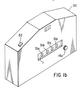
Figure 1b depicts a multi-lens camera with main body 50 containing four imaging lenses 51a, 51b, 51c, 51d. *Id.* at 5:16–18.
