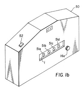
Figure 1b depicts a perspective view of a digital camera with four lenses 51a-51d. Ex. 1007, 5:16-18. Petitioners assert an ordinarily skilled artisan would have understood from Figure 1b that the image sensors corresponding to lenses 51a and 51b are closely positioned with respect to a common plane. Pet. 59 (citing Ex. 1003 ¶ 178).
