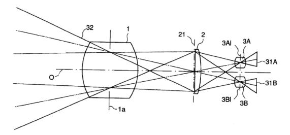
Figure 1 depicts a cross-sectional view of an optical system of one embodiment disclosed by Yamazaki. *Id.* at 3:37–39. In this embodiment, lenses 3A and 3B are positioned behind image sensor elements 31A and 31B. *Id.* at 3:54–60.
